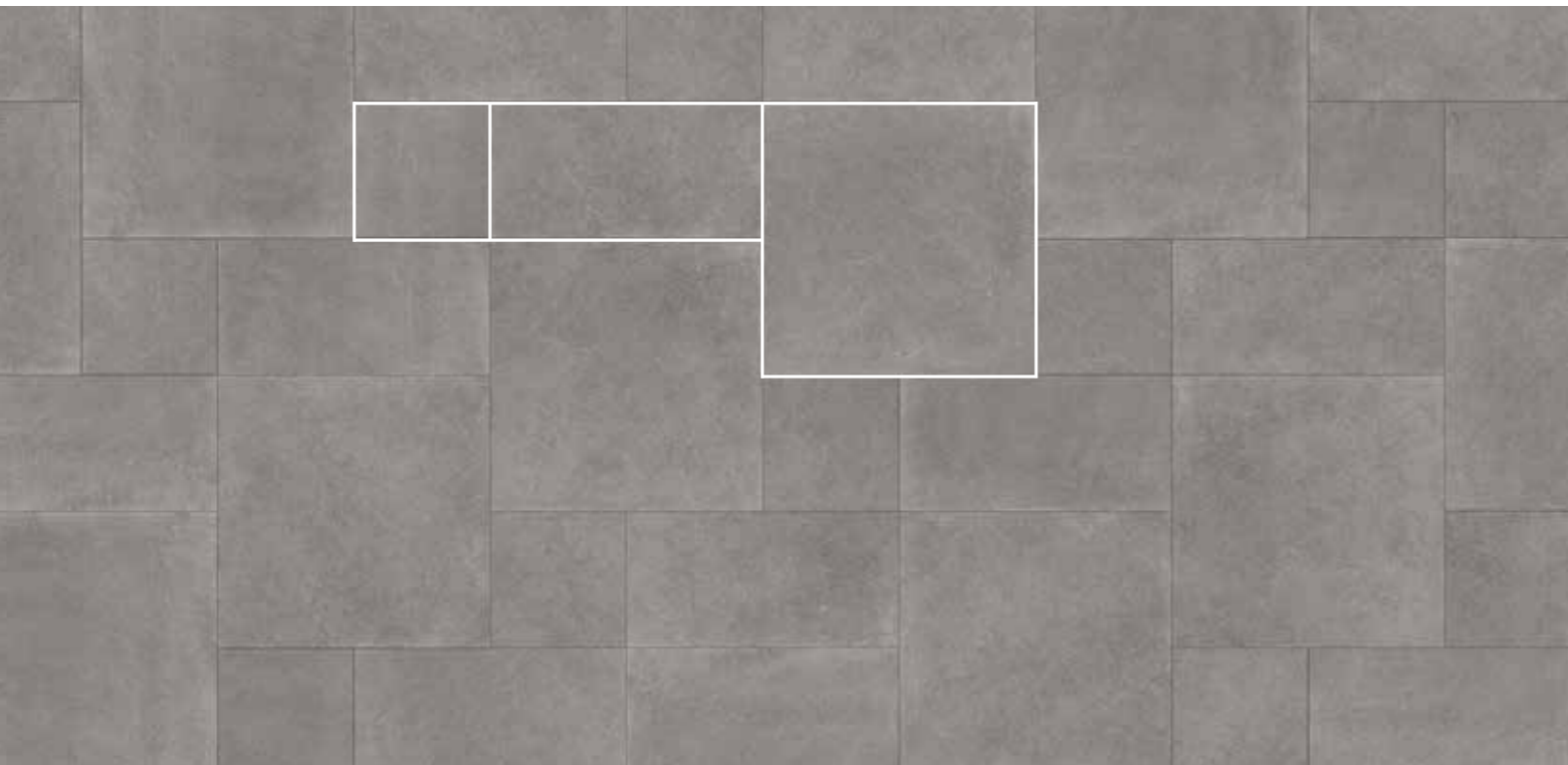
MODULO 3 57% MQ 60x60 24"x24" | 29% MQ 30x60 12"x24" | 14% MQ 30x30 12"x12" - fuga 2 mm
